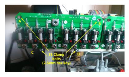
the bottom clamps they should stay pointing downwards due to gravity. Gently puliing from the top 2 corners of the pcb (A,B), remove the T8 unit from the rack unit (with all the wiring still attached).
